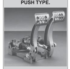
This is a general purpose floor mounted pedal box which utilises the latest high efficiency CP7854 push type master cylinders. Minimum hysteresis and balance variation are assured by the use of needle roller bearings in the centre trunnion and ball bearing pedal
