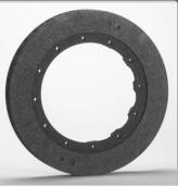
We recommend and supply a number of Hitco Carbon/Carbon materials which we consider to offer the best performance and braking characteristics together with low wear of any material currently available. This section on Carbon discs is designed as a users guide for reference only and we recommend you contact AP Racing technical section for more detailed information before finalising installation details.
