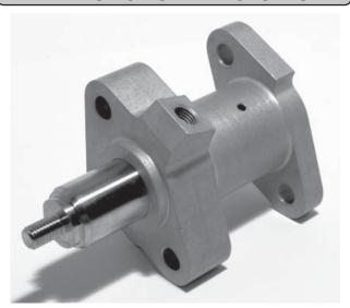
This power actuator is designed to be used in conjunction with an electronic control power hydraulic system (e.g. Paddle Shift) to operate the clutch. It is fitted between the clutch pedal and a standard master cylinder and allows manual operation using the clutch pedal if required.
