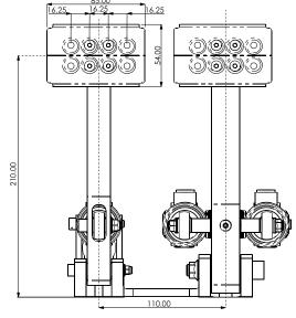
SETTING UP THE BALANCE BAR SELIMIC OF THE BALANCE BAK ADJUST THE PUSHRODS SO THAT THE BALANCE BAR ISPERPENDICULAR TO THE PUSHRODS UNDER MAXIMUM LOAD. THE SYSTEM IS THEN SQUARE. IT IS NOT IMPORTANT THAT THE SYSTEM IS SQUARE WHEN RELEASED, BUT IT HAS TO BE UNDER LOAD.
