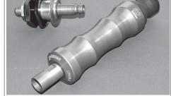
To maintain the lance it is recommended to spray silicone separator. Spray down the nose of the lance and then engage the lance onto the connector for 3 or 4 times to work spray in.
