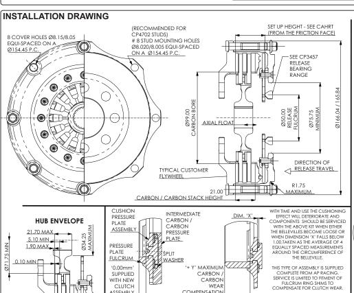
WEAR COMPENSATION IS ACHIEVED BY REPLACING THE PRESSURE PLATE FULCRUM RING AS SHOWN ABOVE. SEE TABLE ABOVE FOR KIT PART NUMBERS AND INCREMENT DETAILS Note: Drawing for guidance only. Download latest issue installation drawing from www.apracing.com
