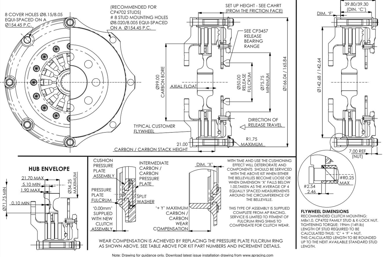
CARBON / CARBON CLUTCH - Ø140mm Push Type - CP6913 & CP6914
