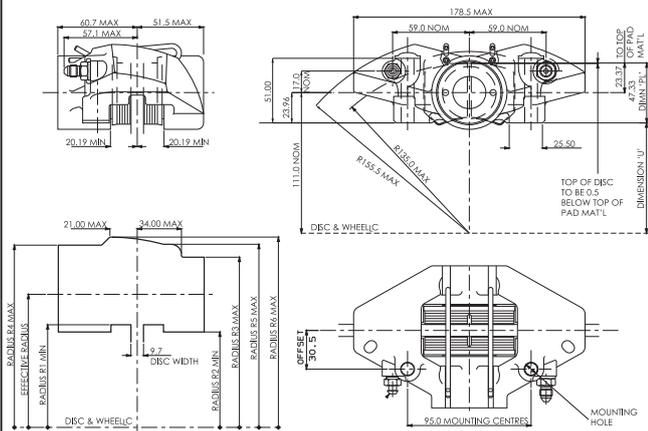
Note: Drawing for guidance only. Download latest issue installation drawing from [www.apracing.com](http://www.apracing.com)
