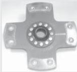
**■ CERAMETALLIC PADDLE:-** Cerametallic buttons riveted to a steel disc giving improved heat dissipation. Used mainly for Rally applications where more clutch slip is required in order to modulate the drive.
