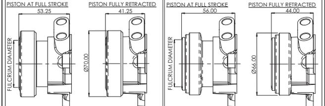
**REDUCED LENGTH - INNER ROTATING RACE BEARING CONFIGURATION 3 (12MM STROKE)** - THIS SLAVE CYLINDER FEATURES: A SHORTENED STROKE SO AS TO REDUCE THE OVERALL LENGTH. THE BEARING HOUSED IN THE PISTON VIA THE OUTER RACE. THE INNER RACE ROTATES, SUITABLE FOR HIGH SPEED APPLICATIONS.
