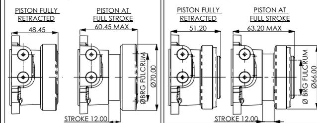
**BEARING CONFIGURATION 3:** The bearing is housed in the piston via the outer race with the inner race rotating. The stroke has been shortened so as to reduce the overall length.
