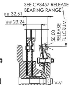
RECOMMENDED CLUTCH MOUNTING (FOR ALL TYPES OF ASSEMBLY M8x1.0 CP4702 STUD FAMILY AND K-LOCK NUT TIGHTENING TORQUE 19Nm (14 lb/ft) LENGTH OF STUD REQUIRED TO BE CALCULATED THUS STUD LENGTH = 'C' + 'F' + ('R' OPTIONAL) + NUT.
