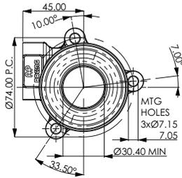
**BEARING CONFIGURATION 1:** The bearing is housed in the piston via the outer race with the inner race rotating. This is more suitable for high speed applications.
