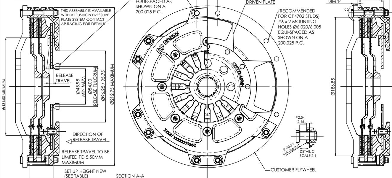
Note: Drawing for guidance only. Download latest issue installation drawing from www.apracing.com
