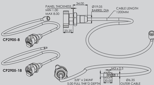
Note: Drawing for guidance only. Download latest issue installation drawing from [www.apracing.com](http://www.apracing.com)
