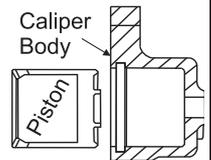
**CP4519 (SEAL IN BORE WITH DIRT SEAL)**
