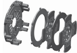
The 'I' Drive design features drive tenons, which locate into internal jaws in the lightweight aluminium clutch cover, eradicating the onset of clutch drag.
