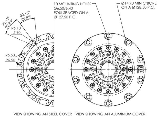
VIEW SHOWING AN STEEL COVER VIEW SHOWING AN ALUMINIUM COVER
