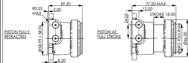
**BEARING CONFIGURATION 2:** The bearing is housed on the piston via the inner race with the outer race rotating. The stroke has been shortened so as to reduce the overall length.
