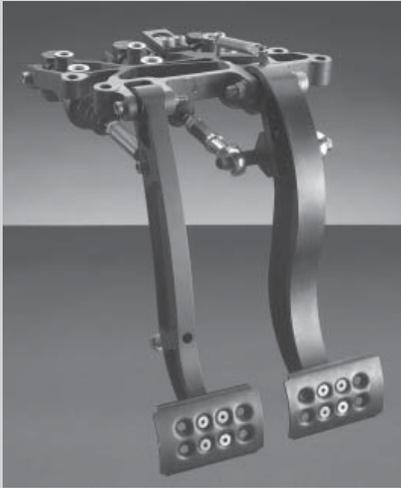
This multi ratio push type pedal box allows the pushrod to remain straight, eliminating all side loads therefore making it very efficient. The master cylinders connect directly to a high efficiency balance bar. A lightweight aluminium base, and ergonomic steel and alloy pedals offer the user the ultimate control in this critical area. Uses CP7854 Master Cylinders.
