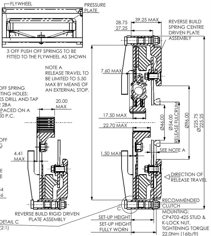
THIS CLUTCH ASSEMBLY IS ONLY SUITABLE FOR USE WITH REVERSE BUILD SPRING CENTRE DEIVEN PLATE ASSEMBLIES
