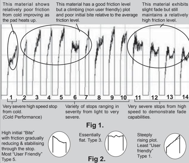
▣ **AVERAGE FRICTION:** Overall mean friction coefficient calculated over the complete test cycle. (Fig 1.)
