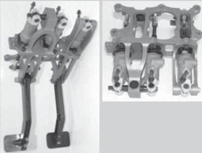
This unique pull type bulkhead mount design with master cylinders being located in the engine or front compartments allows the pushrod to remain in line eliminating all side loads making it one of the most efficient pedal box on the market. It's lightweight aluminium base, and ergonomic steel and alloy pedals offer the user the ultimate control in this critical area.
