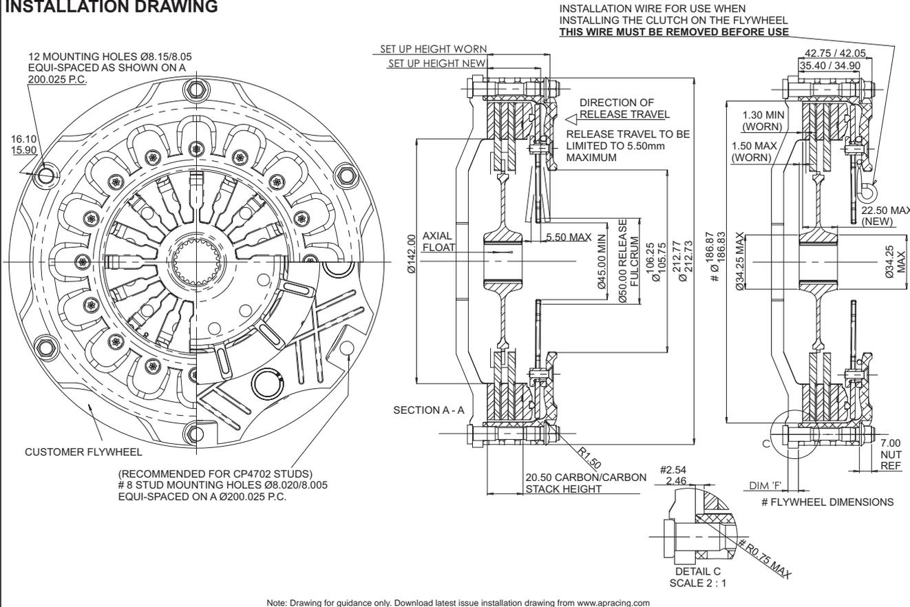
**CARBON / CARBON CLUTCH - Ø200mm Push Type - CP7212 & CP7213**
