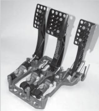
This unique pull type design allows the pushrod to remain in line eliminating all side loads making it the most efficient pedal box on the market. The cylinders are mounted under the drivers feet for optimum space utilisation and access. Minimum hysteresis and balance variation are assured by the use of needle roller bearings in the centre trunion.
