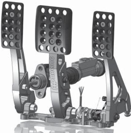
CP5540-50 is a floor mounted push type racing pedal box, incorporating a tandem master cylinder CP5540 family for brake application only and a standard cylinder is required for clutch actuation. The tandem master cylinder removes the ability to adjust the brake balance during an event, therefore brake balance should be set by selecting an appropriate bore within the master cylinder range.
