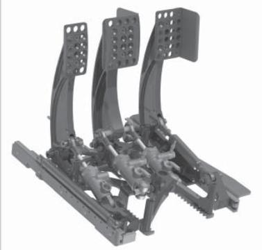
This unique optimised pull type sliding pedal box is AP Racing's solution to comply with the potential new safety regulation of a fixed driver seat in GT Racing allowing for the accommodation of different height drivers in the same car.
