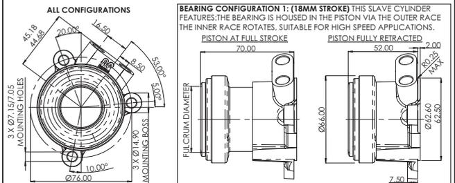
**BEARING CONFIGURATION 1: (18MM STROKE)** THIS SLAVE CYLINDER FEATURES: THE BEARING IS HOUSED IN THE PISTON VIA THE OUTER RACE THE INNER RACE ROTATES, SUITABLE FOR HIGH SPEED APPLICATIONS.
