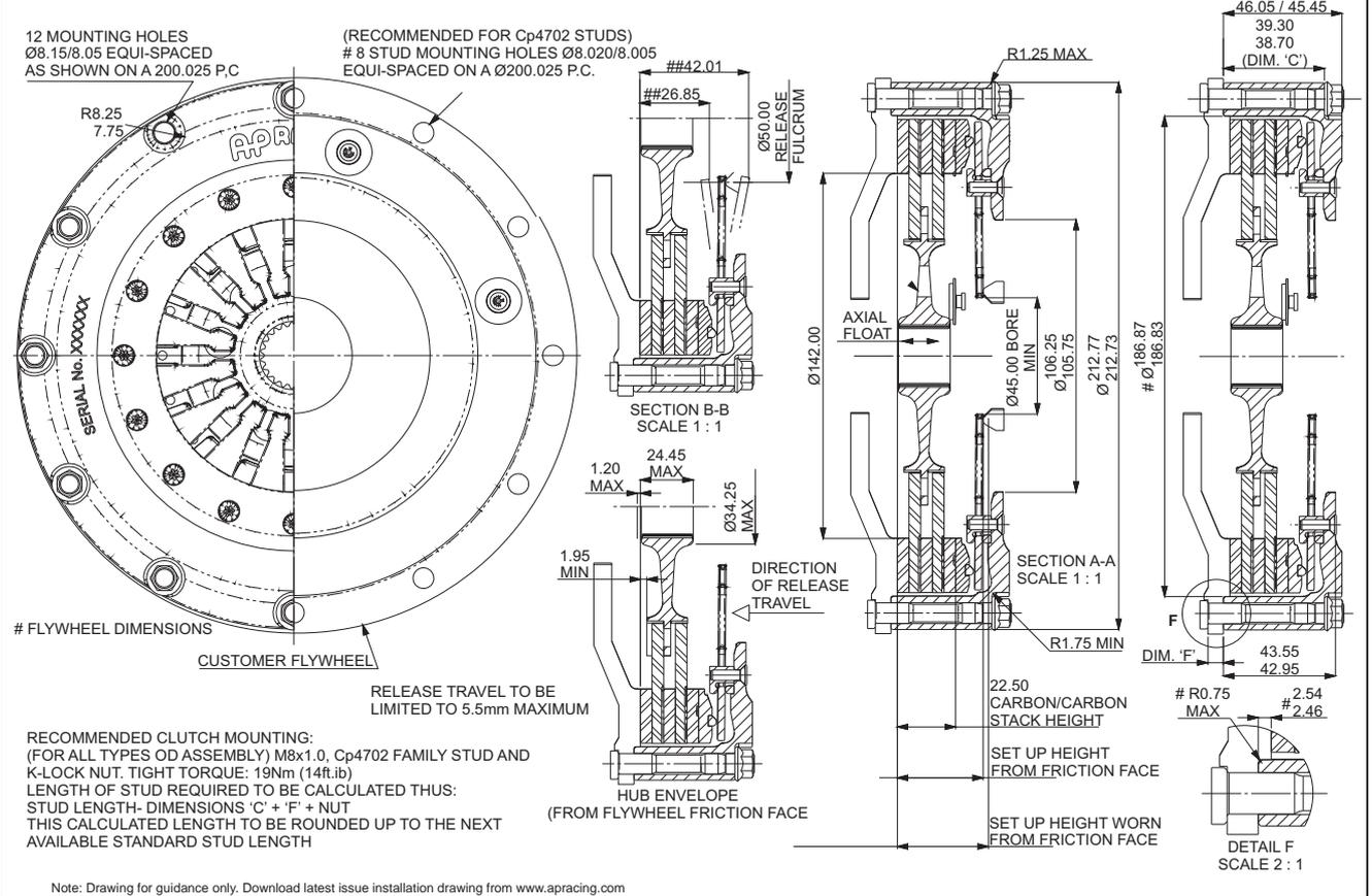
**CARBON / CARBON CLUTCH - Ø184mm Push Type - CP8792**
