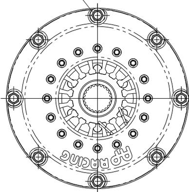
THE CLUTCH SPIGOT HAS BEEN DESIGNED TO BE THIS DIAMETER WHEN BOLTED TO THE FLYWHEEL BEFORE FITTING (WITH THE INSTALLATION WIRE IN PLACE) THIS DIAMETER MAY BE SLIGHTLY REDUCED
